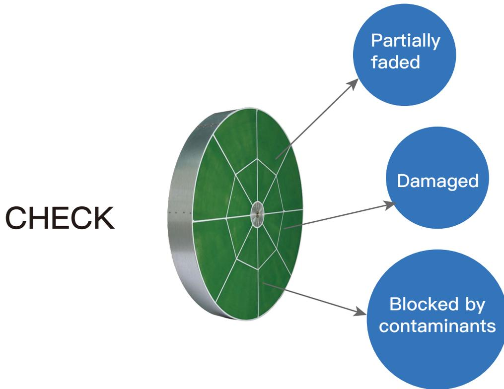
Carefully check whether the surface of the wheel is partially faded, damaged, or blocked by contaminants. It indicates that the wheel has been damaged by high temperature if the surface color changes to a different color. The heating temperature should not exceed the temperature which the wheel can withstand.
